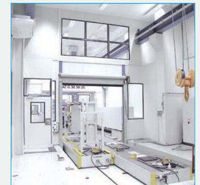
Moving of parts on air cushion system
